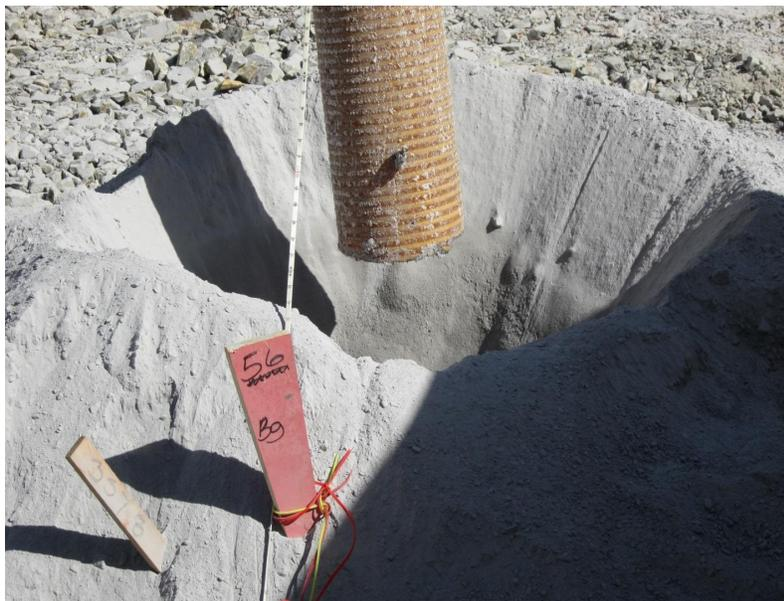
Photo No. 1: Close-up of Drill Cuttings around Blasthole
