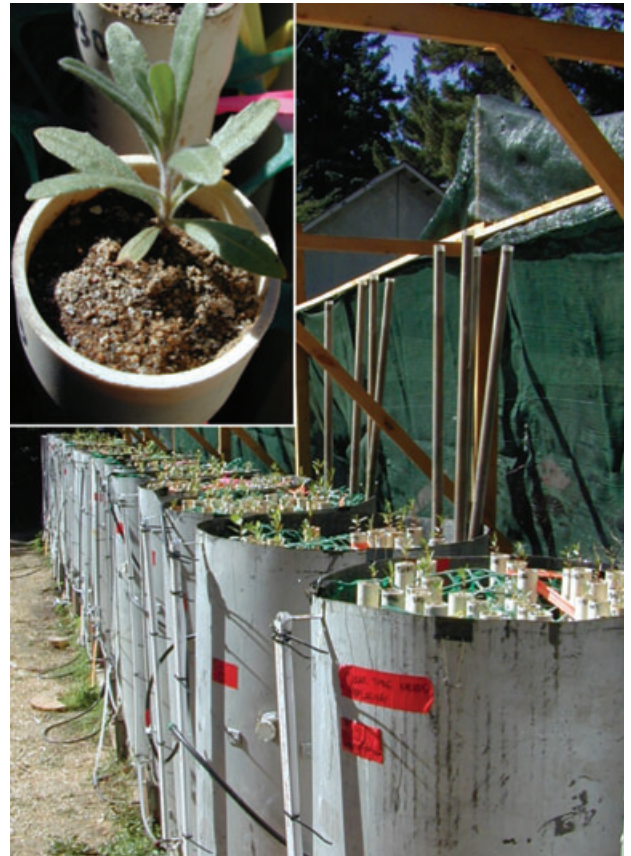
Figure 1. The experimental setup consisted of 20 tanks with seedlings grown in PVC tubes suspended within each tank (inset). Four tanks were randomly assigned to each of five drawdown treatments. Each tank contained individuals of all species tested.
