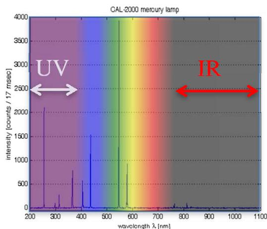
*Spectrum of mercury vapor lamp typically used for streetlighting.*
